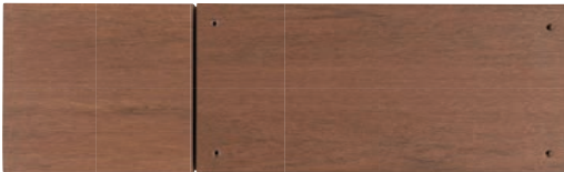
Weathered TimberTech Advanced PVC after 6 months
