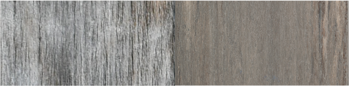
Wood Weathered Ipe after 5 years TimberTech Coastline
